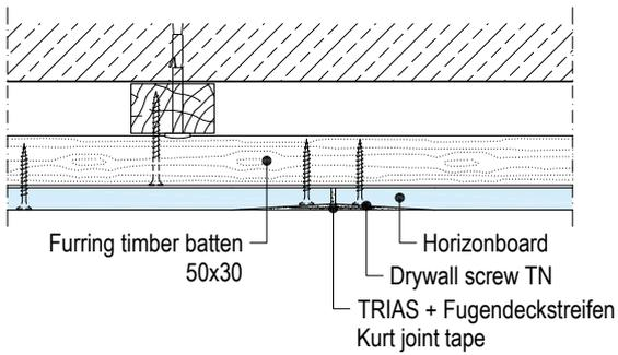
**D111.de-C5 Front edge – Horizonboard**
