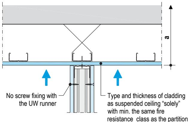
Partitions with the same fire resistance class as the entire ceiling system (a) must be fastened to the basic ceiling.
