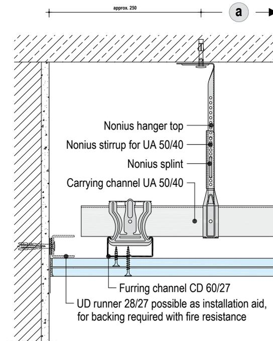
D116.de-B1 Longitudinal edge – Carrying channel/furring channel/Nonius stirrup
