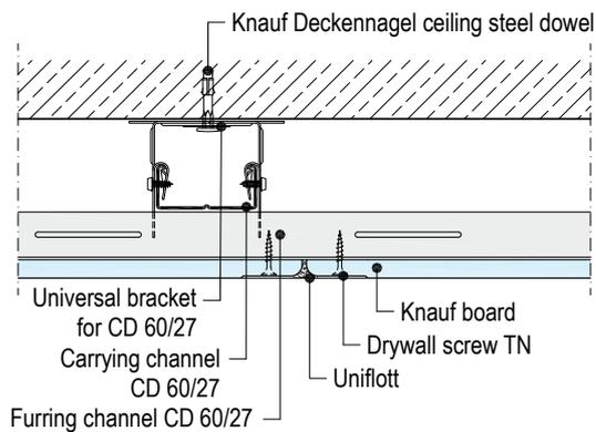
D112.de-C2 Front edge – Carrying channel/furring channel/universal bracket
