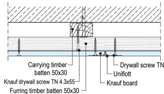
D111.de-C1 Front edge – Carrying channel/furring batten/directly anchored
