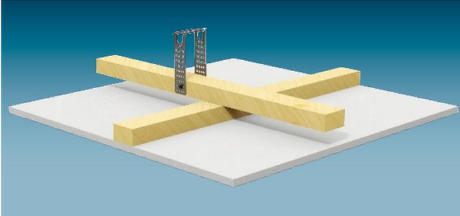
Knauf boards are fixed with screws to a wood frame made of carrying timber battens and furring timber battens (double batten frame) or just simple furring timber battens (single batten frame).
