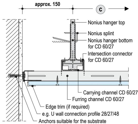
D112.de-A4 Connection to wall with face joint
