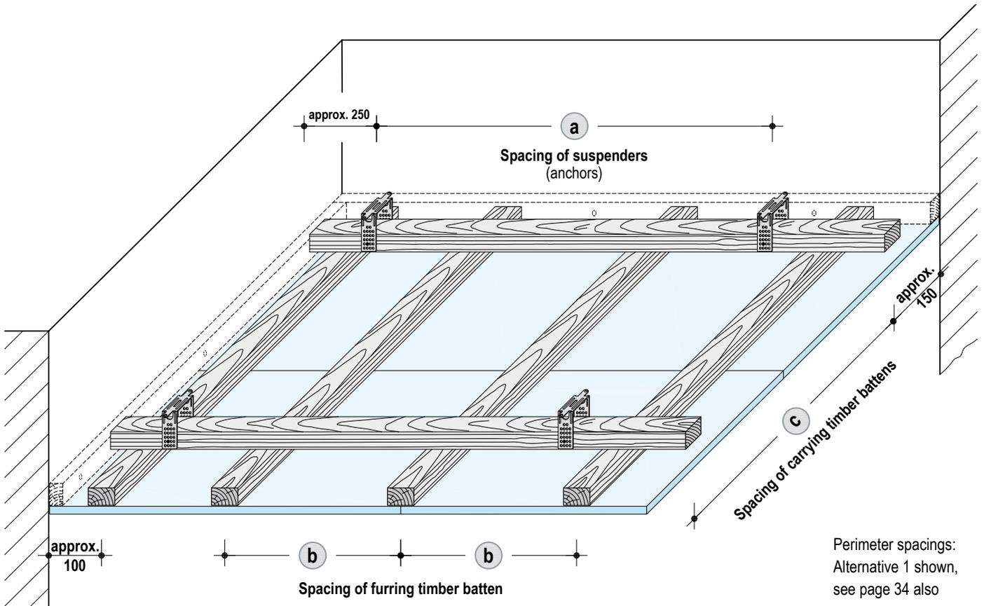
**Without fire resistance** – carrying timber batten and furring timber batten  $\geq 50 \times 30$  mm
