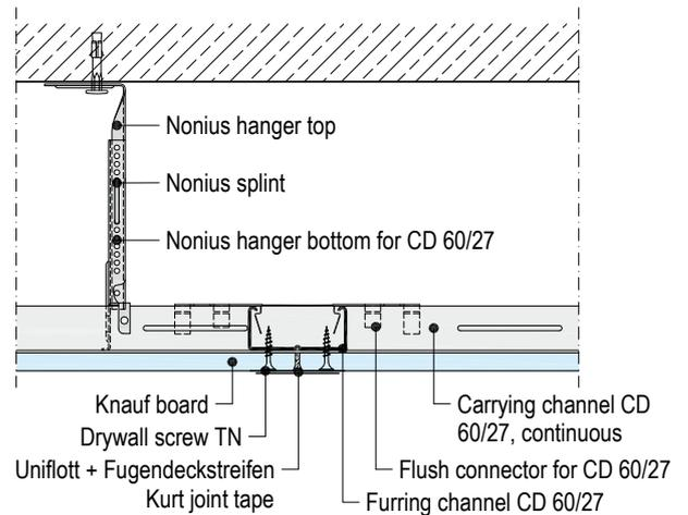
**D113.de-B4 Connection of lightweight partition to ceiling**
