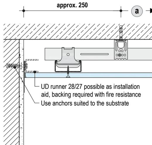
D112.de-B2 Longitudinal edge – Carrying channel/furring channel/universal bracket
