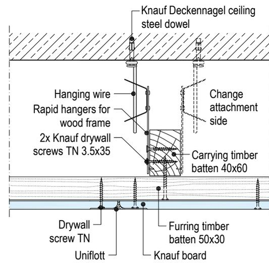
**D111.de-C4 Front edge – Carrying channel/furring batten/rapid hanger**
