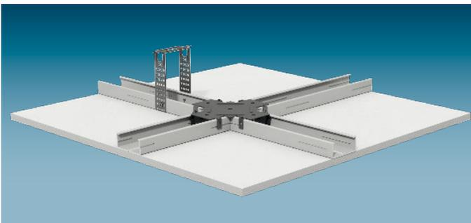
Knauf boards are fixed with screws to a metal grid of flush carrying and furring channels made of sheet metal profiles CD 60/27.
