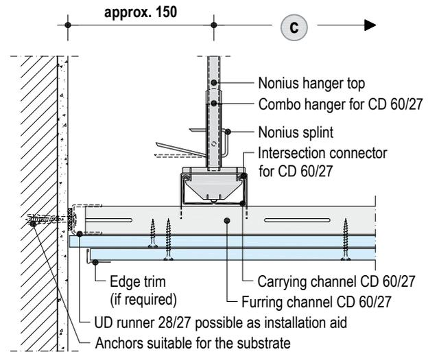
D112.de-D4 Connection to wall with shadow gap
