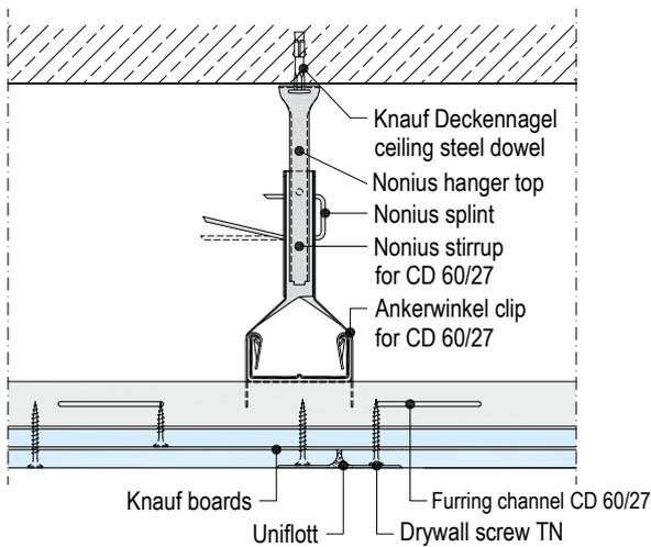
D112.de-C1 Front edge – Carrying channel/furring channel/Nonius stirrup
