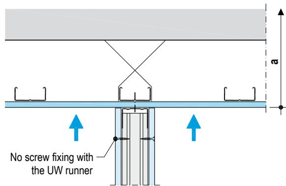
If partitions with fire protection requirements are connected to the suspended ceiling, the classification of the suspended ceilings alone must at least be the same fire resistance class as the partition.
