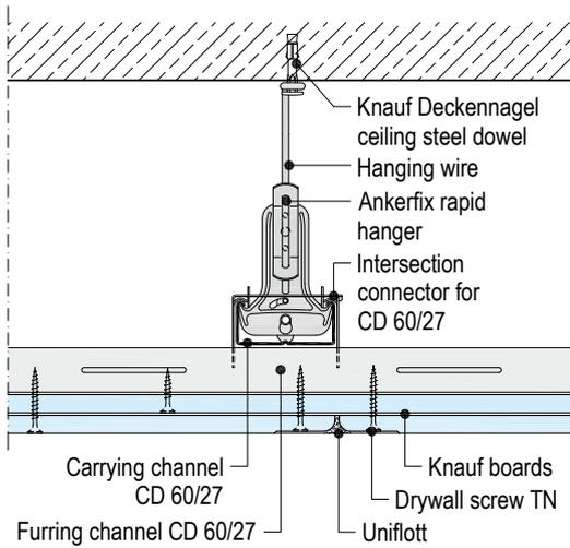
D112.de-C4 Front edge – Carrying channel/furring channel/Ankerfix
