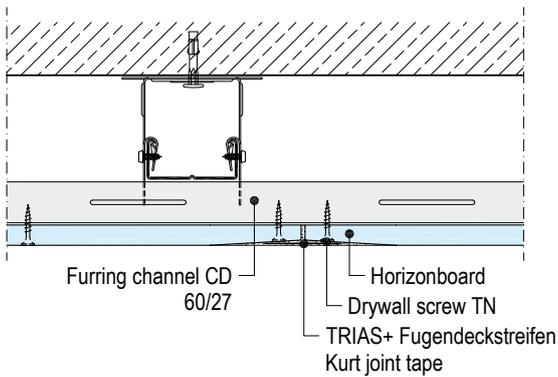
**D112.de-C8 Front edge – Horizonboard**
