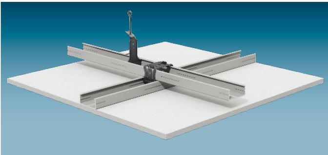
Knauf boards are fixed with screws to a metal grid made of carrying and furring channels (double layer profile) or just furring channels (single layer profile) made of sheet metal profiles CD 60/27 or hat-shaped channels.
