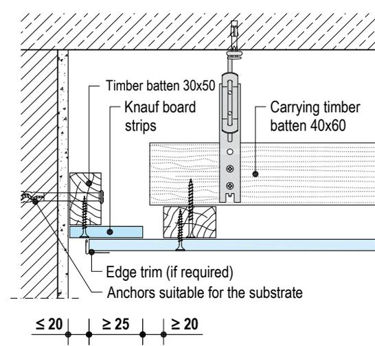
**D111.de-B2 Longitudinal edge – Carrying channel/furring batten/rapid hanger**
