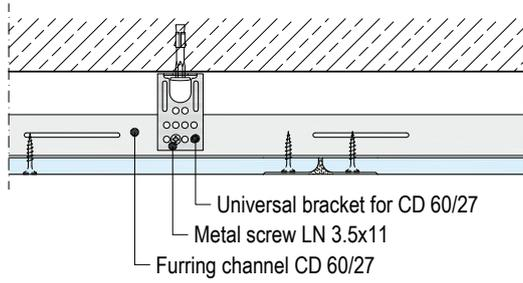
**D112.de-C9 Front edge – Furring channel/Ankerfix**
