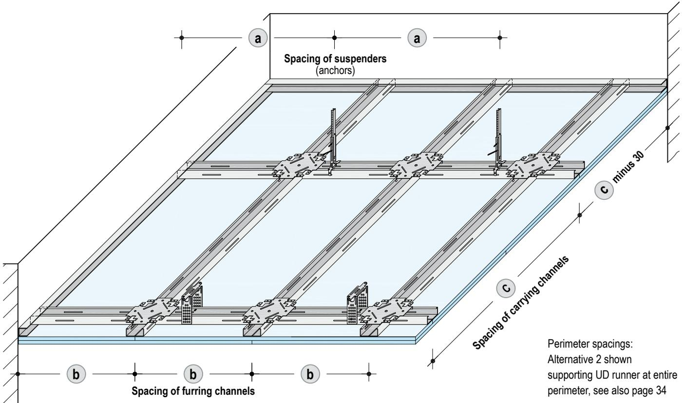
Without fire resistance/fire resistance solely from below – carrying and furring channel
