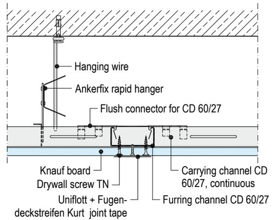
**D113.de-B5 Longitudinal edge – flush/Nonius hanger**
