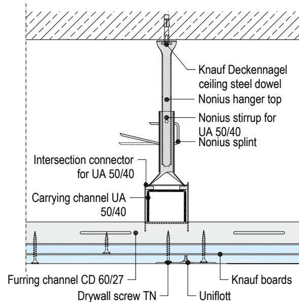
D116.de-C1 Front edge – Carrying channel/furring channel/Nonius stirrup
