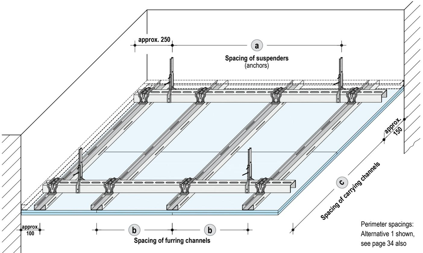
Without fire resistance/fire resistance solely from below – carrying and furring channel
