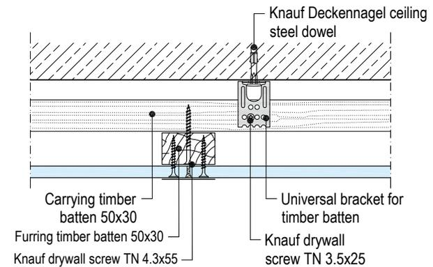
D111.de-B4 Longitudinal edge – Carrying channel/furring batten/ directly anchored
