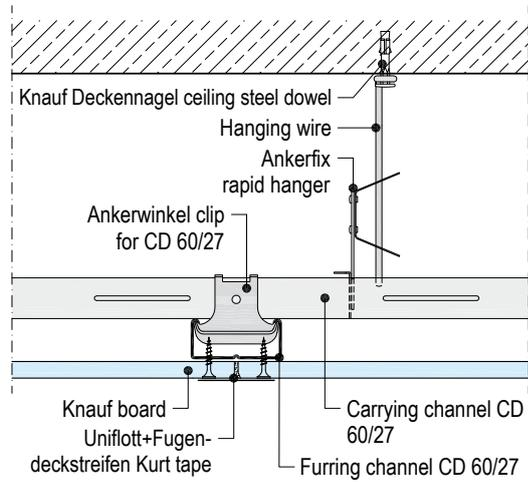
D112.de-B1 Longitudinal edge – Carrying channel/furring channel/Nonius stirrup
