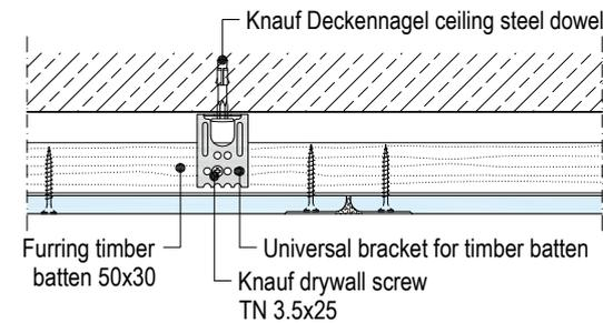
D111.de-C2 Front edge – Carrying channel/furring batten/ universal bracket
